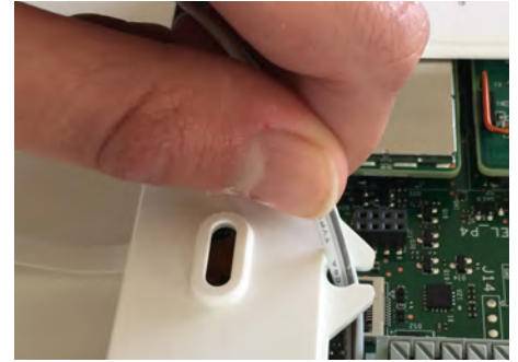
Insert the wire into the strain-relief
