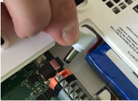
Plug in the power connector
