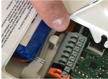
Route the wire behind the retainer clip
